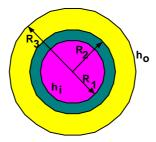
R<sub>1</sub> and R<sub>2</sub> are the inside and outside radius of the pipe.
